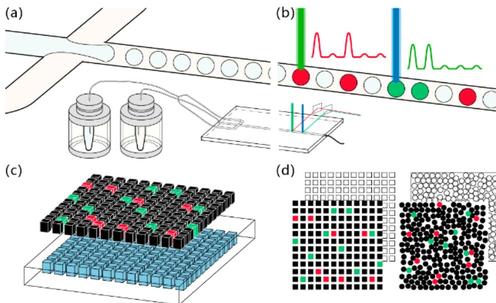
**Figure 2.** Microfluidic digital PCR partitioning and counting strategies. (a) Emulsion droplet generation using flow-focusing microfluidic chip; (b) Serial droplet fluorescence reading; (c) Minute volumes of PCR sample are partitioned in micro-well microfluidic chip; (d) Planar imaging for fluorescence positive chamber counting.
