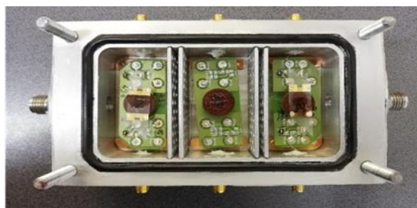
Figure 1. Surface Acoustic Wave (SAW) sensors in the test chamber.
