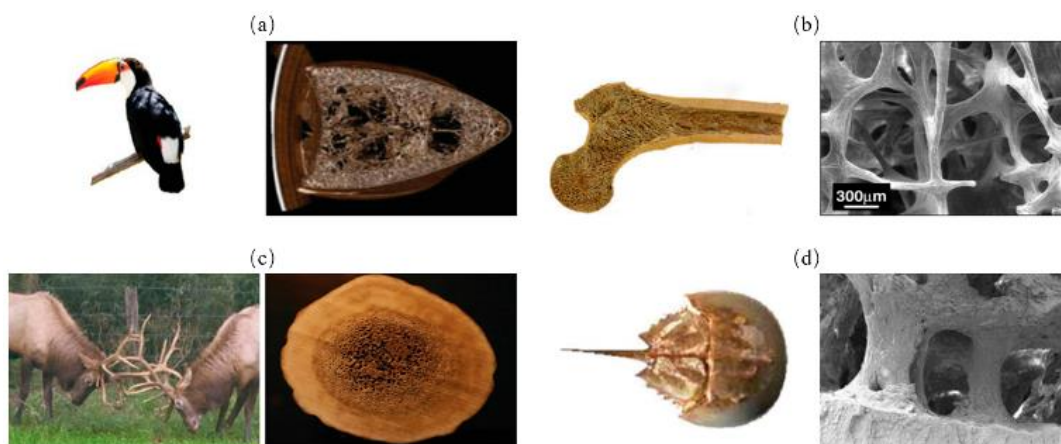
Figure 12. Sandwich model in biological organisms. (a) toucan beak [62] Copyright©2005, Acta Materialia (b) human trabecular bone [51] Copyright©2007, Progress in Materials Science (c) antler [63] Copyright©, 2010Acta Biomaterialia. (d) horseshoe crab [64]. Copyright©2018, Progress in Materials Science.
