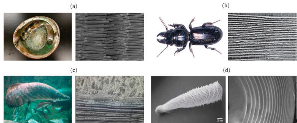
Figure 2. Layered model in biological organisms. (a) nacre shell [24] Copyright©2009, Progress in Materials Science (b) beetle shell [25] Copyright©2008, Advanced Engineering Materials (c) fish scale [26] Copyright©2012, Journal of Materials Research (d) concentric layer of deep-sea sponge [27] Copyright©2008, Journal of Materials Research.
