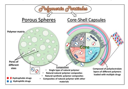
Figure 2. Structural configurations of core-shell and porous natural polymeric/protein particles.
