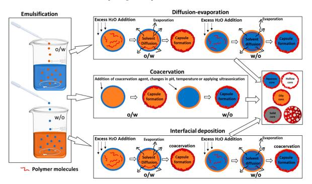
Figure 4. Schematic diagram of emulsion templating approach.
