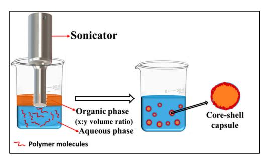
Figure 5. Schematic diagram of ultrasonication-assisted emulsification-coacervation.
