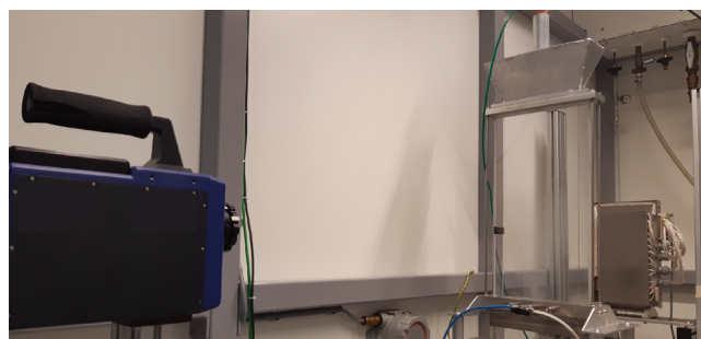
Figure 1. Experimental setup consisting of the IR source on the right, quartz glass column in the middle, and IR camera on the left.
