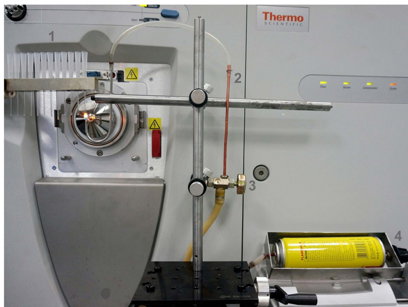
Figure 1. The photograph of ambient flame ionization mass spectrometry (AFI-MS) apparatus for direct analysis of the sample. 1. sample rods, 2. butane transferring pipe, 3. flow micro-adjust valve, 4. pressure controlling valve. The analytes could be desorbed and ionized rapidly in the outer flame region, and the ions generated by AFI could be transferred and detected by the mass spectrometry. The optimal distance between the centre of flame and the inlet to mass spectrometer is 10 mm. The ideal size of butane flame (height about 1 cm) is controlled by pressure controlling valve and exactly adjusted by flow micro-adjusting valve.
