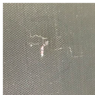
Figure 13. Surface cracks after impact.
