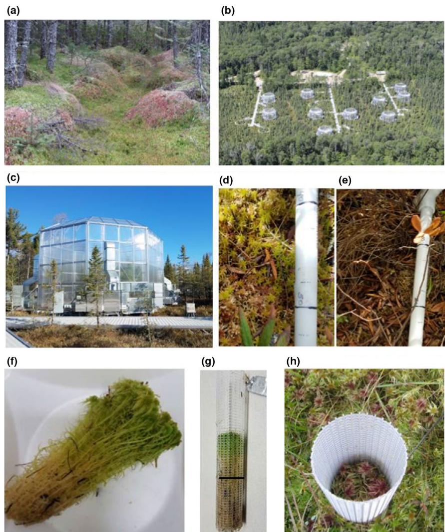
FIGURE 2 SPRUCE experiment layout. (a) Hummocks and hollows with Sphagnum mosses beneath Picea mariana trees. (b) Ten whole-ecosystem enclosures, isolated from one another and distributed in a bog in northern Minnesota, USA. (c) Open-top enclosure. (d, e) Guides for community composition assessments. (d) Mixture of S. magellanicum and S. angustifolium . (e) Dead Sphagnum beneath shrub litter. (f) Clump of Sphagnum cut to 7 cm length and ready for insertion into a plastic mesh column. (g) The column after removal from the field one year after deployment; the black line indicates the height of the Sphagnum . (h) The mesh column for measuring dry matter production inserted into the plot
