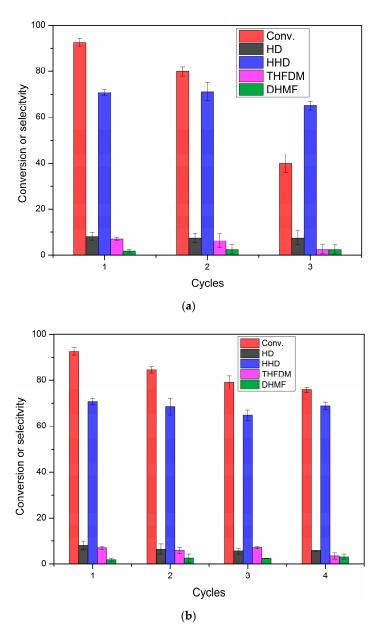
**Figure 4.** Reuse experiment for the hydrogenation of HMF to HHD with different recycling method, washed by  $H_2O/C_2H_5OH$  (a), further washed in hot tetrahydrofuran (b). Reaction conditions: Pd/C (12.5 mg, mole ratio, HMF/Pd = 420:1), HMF (2.5 mmol), AcOH (60.0 mg, 1 mmol),  $H_2O$  (2.00 g),  $H_2$  (4 MPa), 393 K, 3 h. The error bars refer to the confidence interval with 95% confidence.
