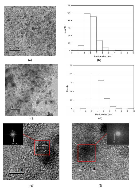
**Figure 6.** TEM images, the particle size distribution and HRTEM images of fresh Pd/C (a,b,e) and the used Pd/C (c,d,f). The inset in the HRTEM image is the diffraction spots after fast Fourier transform.
