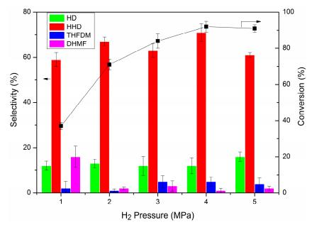
**Figure 1.** The effect of  $H_2$  pressure on the hydrogenation of HMF. Reaction conditions: Pd/C (5.0 mg, mole ratio, HMF/Pd = 420:1), HMF (1 mmol), AcOH (60.0 mg, 1 mmol),  $H_2O$  (2.00 g),  $H_2$  (1–5 MPa), 393 K, 1 h. The error bars refer to the confidence interval with 95% confidence.
