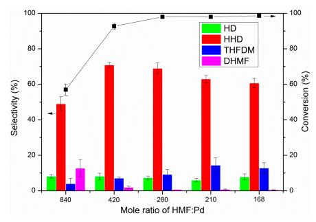
**Figure 3.** The effect of mole ratio on the hydrogenation of HMF. Reaction conditions: Pd/C (12.5 mg, mole ratio, HMF/Pd = 420:1), HMF (2.5 mmol), AcOH (60.0 mg, 1 mmol),  $H_2O$  (2.00 g),  $H_2$  (4 MPa), 393 K, 3 h. The error bars refer to the confidence interval with 95% confidence.
