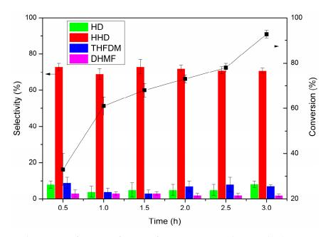
**Figure 2.** Hydrogenation of HMF as a function of time. Reaction conditions: Pd/C (12.5 mg, mole ratio, HMF/Pd = 420:1), HMF (2.5 mmol), AcOH (60.0 mg, 1 mmol),  $H_2O$  (2.00 g),  $H_2$  (4 MPa), 393 K, 0.5–3 h. The error bars refer to the confidence interval with 95% confidence.
