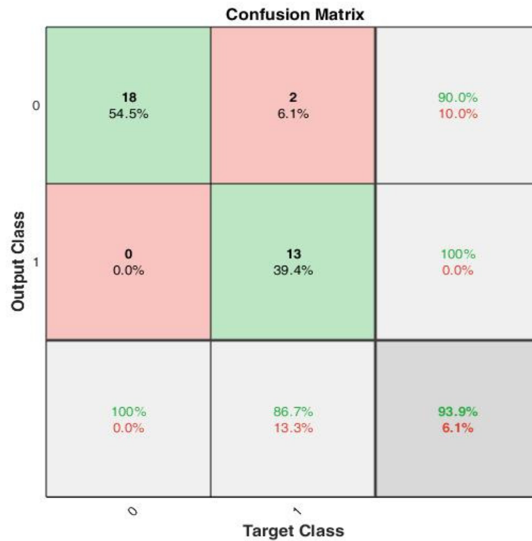
Figure 8. A confusion matrix that summarizes the model performance with true positivity rate and true negativity rate, with accuracy of 100%, 90% and 93.9%, respectively.
