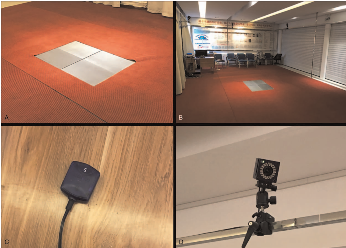
Figure 2. Spatial layout of 3D dynamic capture device. (A) Four three-dimensional force plates were embedded in the vertical direction in the ground, (B) the gait analysis room, (C) the surface EMG device and (D) optical cameras. 3D = three-dimensional, EMG = electromyogram.
