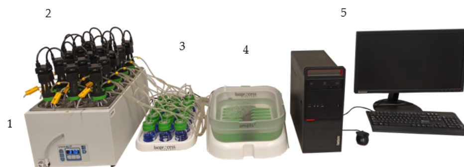
Figure 2. Biochemical methane potential test equipment AMPTS II, 1—water bath, 2—reactors with agitation, 3—CO 2 absorption units, 4—gas volume meters, 5—computer.
