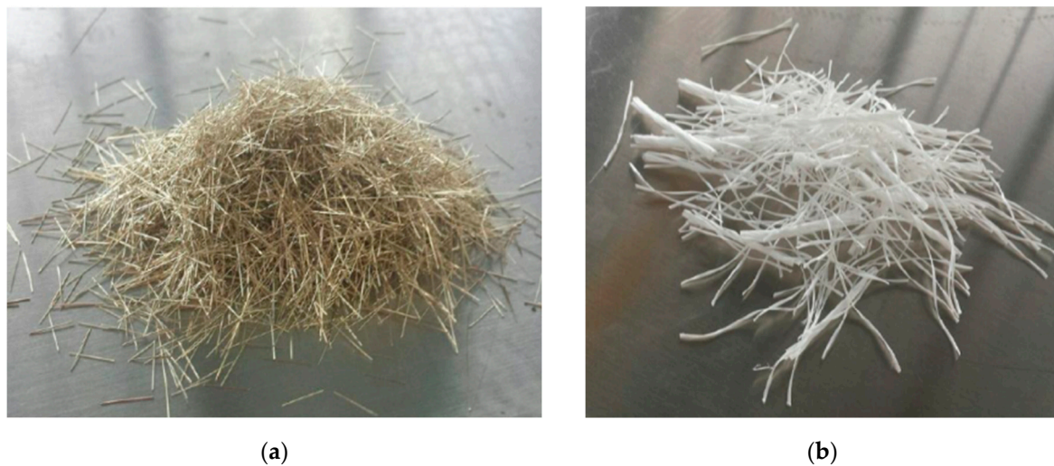
Figure 1. Type of fibers used in conducted studies: (a) steel fibers and (b) polypropylene fibers.
