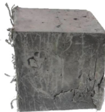
Figure 8. Destroyed fiber-reinforced concrete with polypropylene fibers (F-RCP) cubic specimen after the strength test.
