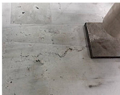
Figure 17. Compression zone of the damaged C-REF + fiber-reinforced concrete with steel fibers (F-RCS) slab element.
