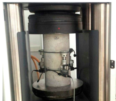
Figure 3. Test setup for testing the static modulus of elasticity of reference concrete (C-REF).
