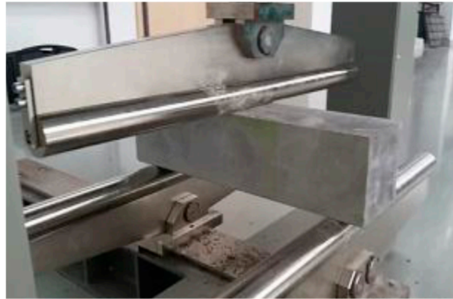
Figure 4. Flexural strength test of C-REF.
