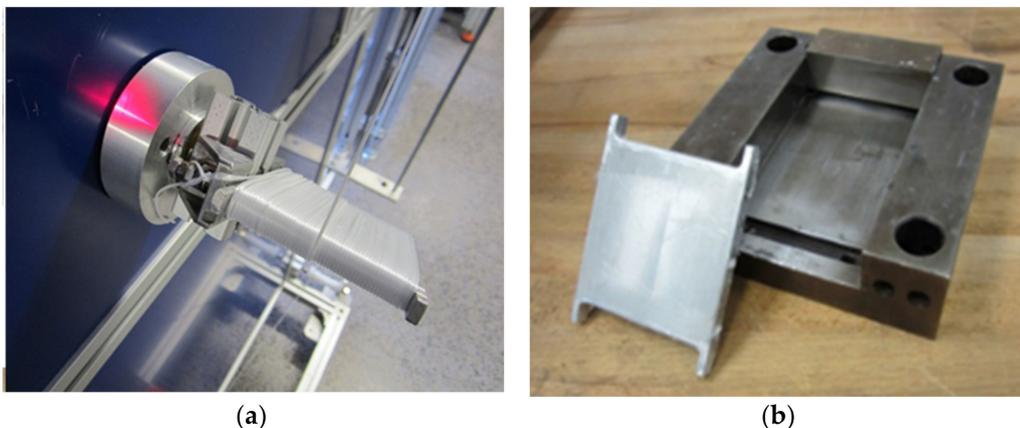
**Figure 1.** Production of MFC composite plate, (a) filament winding around the aluminum plate, (b) compression hot press mold.
