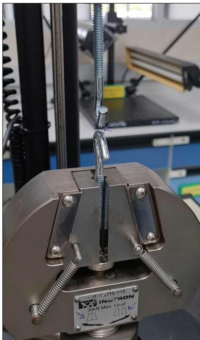
Figure 2: Mounted suture sample with metal hooks on the Universal Testing Machine
