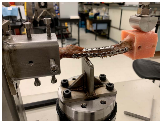
Fig. 3 For the nondestructive bending tests, the medial end of the clavicle was perpendicular to the actuator. The force was applied at the lateral PMMA-potted end of the clavicle, with the actuator 10 cm lateral to the fulcrum.
