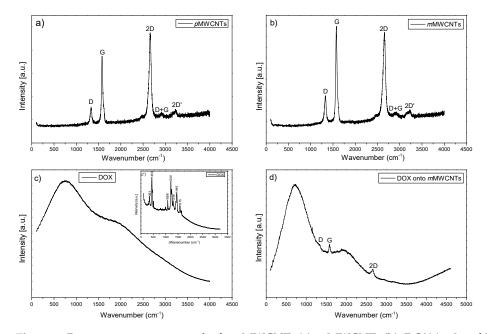
**Figure 2.** Raman spectroscopy results for *p*MWCNTs (**a**), *m*MWCNTs (**b**), DOX (**c**,**c**') and DOX onto *m*MWCNTs (**d**).
