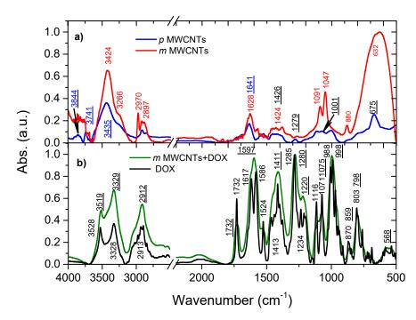
**Figure 1.** FTIR comparison of: *p*MWCNTs and *m*MWCNTs (**a**) and DOX and DOX onto *m*MWCNTs (**b**).
