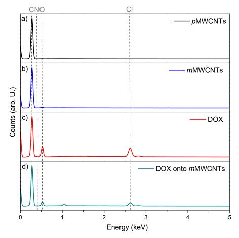
**Figure 4.** EDS spectra of *p*MWCNTs (**a**), *m*MWCNTs (**b**) doxorubicin (**c**) and doxorubicin adsorbed onto *m*MWCNTs (**d**).
