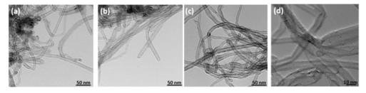
**Figure 5.** TEM images of pristine MWCNTs (**a**), chemically modified MWCNTs (**b**) and chemically modified MWCNTs with adsorbed doxorubicin (**c**,**d**).
