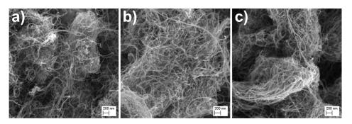
Figure 3. SEM images of (a) *p*MWCNTs (b) *m*MWCNTs and (c) *m*MWCNTs with adsorbed DOX.
