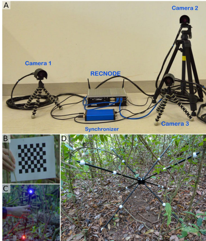
Fig. 2. Example multi-camera recording system. (A) The three cameras on tripods are connected to a central computer (“Recnode”) and a hardware synchronizer. (B) Checkerboard used for intrinsic calibrations and (C) Wands with two different light sources used for extrinsic calibration of cameras. (D) Multi-armed structure for ground-level calibration, with known distances between white balls and a spirit level in the center (see section “Camera calibration” for more detail).
