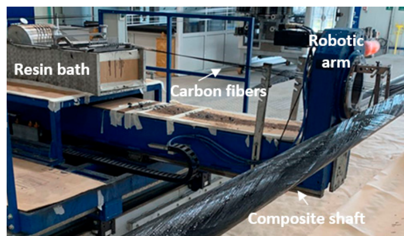
Figure 1. Filament winding system for fabrication of carbon fiber-reinforced polymer (CFRP) shafts.
