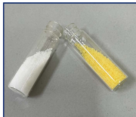
Fig. 16 Silica gel showing the colorimetric response of L (100 \mu\text{M} in acetonitrile) towards \text{Cu}^{2+} ions in a solid medium.
