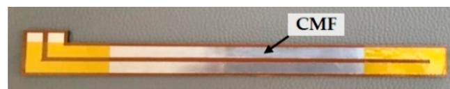
Figure 12. Specimen with conventional metal film (CMF) affixed on the surface.
