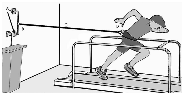
Figure 3 A runner fitted with a leather weightlifting belt (D) attached with a rigid tether (C) to the wall-mounting bracket (A and B) sprinting on a motorised treadmill.
