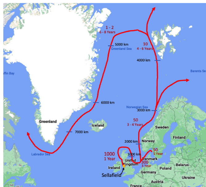
Fig. 9. Ocean transport of ^{137}\text{Cs} to the Arctic. The numbers in bold indicate the concentrations of ^{137}\text{Cs} , relatively to a maximum level of 1000 at the primary source. The years indicate the duration of transport, and the distance from the source (in km) is given.
