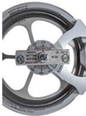
Figure 6. Depth control (top view).
