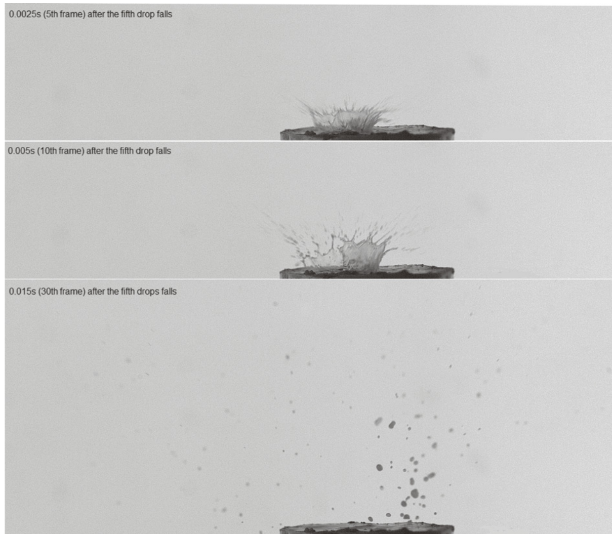
Fig 2. The dependence of the course of time (5 th , 10 th and 30 th frames) of the splash phenomenon after the 5 th drop falls.
