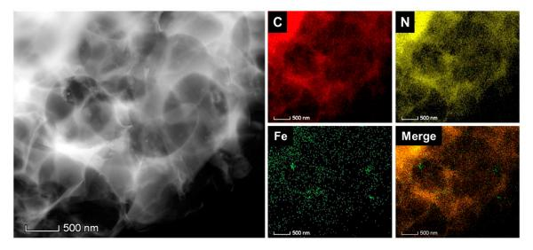
**Figure 3.** High-angle annular dark-field scanning TEM (HAADF-STEM) image and EDS elemental mapping images of PB@PCM for carbon ©, nitrogen (N), and iron (Fe). PB particles uniformly distributed over the whole PCM surface.
