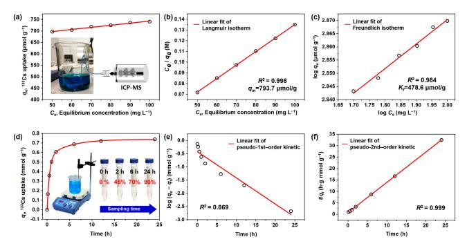
**Figure 5.** (a)  $^{133}$ Cs ion uptake behavior as a function of equilibrium ion concentration and adsorption isotherms for  $^{133}$ Cs ion uptake by the PB@PCM, linearly fitted to the (b) Langmuir and (c) Freundlich isotherm equation. (d)  $^{133}$ Cs ion uptake behavior as a function of contact time and adsorption isotherms for  $^{133}$ Cs ion uptake by the PB@PCM, linearly fitted to (e) pseudo-first-order and (f) pseudo-second-order kinetics.
