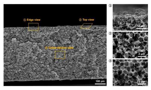
Figure 2. FE-SEM images of the 3D porous carbon monolith at different sections (edge, top, cross-section).
