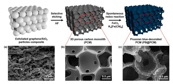
**Figure 1.** A schematic illustration for fabricating PCM through etching of the silica particle templates in EG/SiO<sub>2</sub> composite and obtaining PB@PCM by a subsequent decoration of PB nanoparticles into the PCM. FE-SEM images of (a) EG/SiO<sub>2</sub> particles composite, (b) PCM, and (c) PB@PCM.
