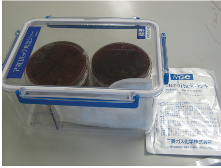
FIGURE 1: Anaerobic jar (left) and anaerobic gas-producing pouch (right). An opened pouch and blood agar plate are inside the jar.
