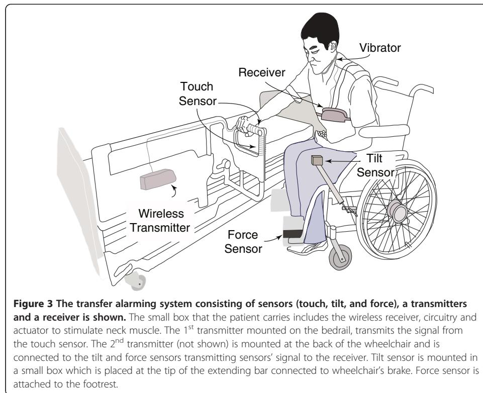
illumination stimulation is produced. For the neck muscle vibration stimulation, the actuator vibrates the patient's neck muscle. LEDs mounted on top of the brake illuminate for light stimulation. Multiple outputs of the system are also possible. For example, the combination of neck muscle vibration with LEDs illumination stimuli is possible.
