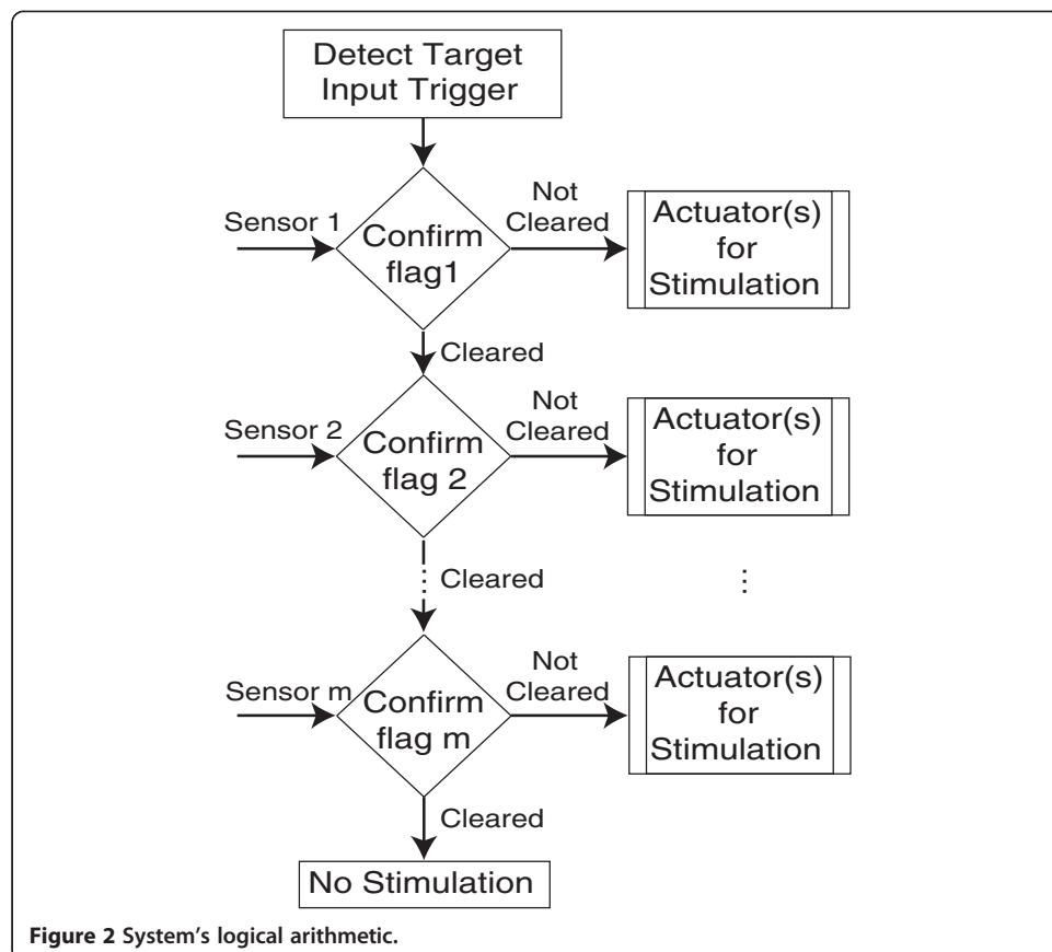
mounted on a footrest of the wheelchair. The actuators are voice alarming, neck muscle vibration and LEDs illumination on the top of the brake of the wheelchair. The case of stimulation for neck muscle vibration is shown in Figure 3.
