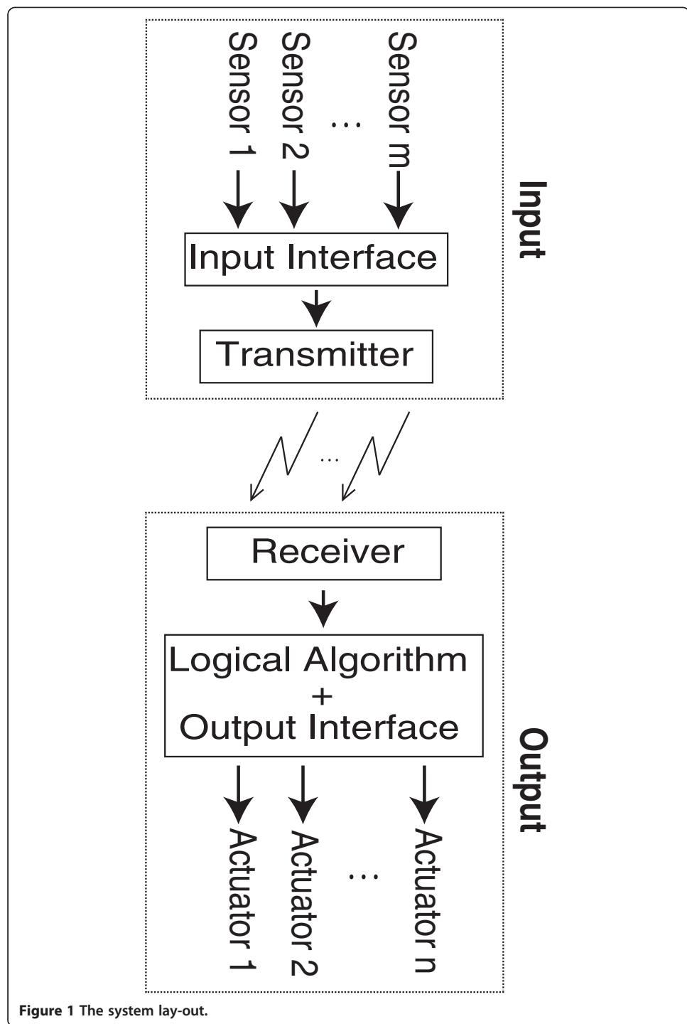
Figure 1 The system lay-out.
