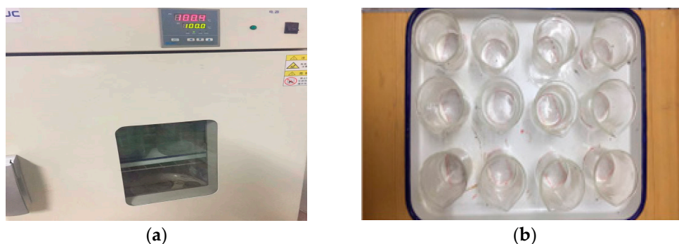
Figure 5. The evaporation test. ((a) DHG-9140a, (b) The counting cup).
