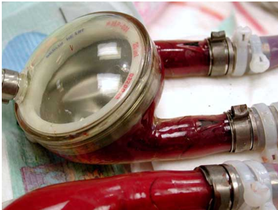
Fig. (2). The Berlin Heart VAD (Berlin Heart AG, Berlin, Germany) consists of a paracorporeal, pneumatically driven pump. The pump is made of a translucent, semirigid housing of polyurethane divided into a blood chamber and an air chamber by a three layer flexible diaphragm.
