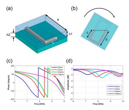
**Figure 2.** The element design and its simulation performance. (**a**) The detailed structure of the metasurface element. (**b**) The liquid-metal reconstruction by rotating the element. (**c**) The simulated results of reflection phase responses of four element dimensions, where d is 6.6 mm, 9.2 mm, 8.04 mm, 7.65 mm. (**d**) The simulated results of reflection amplitude responses of four element dimensions, where d is 6.6 mm, 9.2 mm, 8.04 mm, and 7.65 mm.
