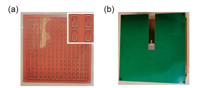
**Figure 4.** The fabricated metasurface antenna sample photograph. (**a**) Photograph of the liquid-metal metasurface sample as well as its enlarged figure of the element. (**b**) The assembled metasurface antenna fed by a micro-strip antenna.
