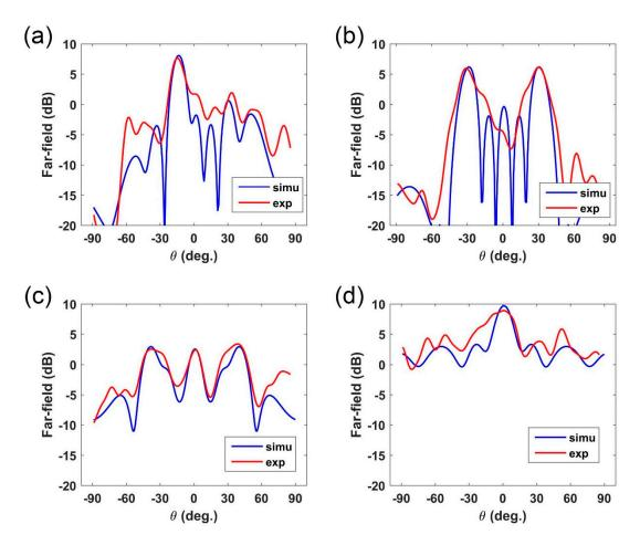
**Figure 5.** The measured far-field results for the designed four-phase distributions, as well as the related simulation data for comparison. (**a**–**c**) The measured far-field results for plane-wave incidence to realize one-beam, dual-beam, and three-beam. (**d**) The single beam reflection under antenna excitation.
