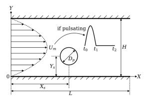
**Figure 3.** Configuration of a particle migrating in Poiseuille channel flow. The origin coordinate locates at left down corner, X in horizontal direction and Y in vertical direction. The simulation domain size is fixed as  $L \times H$ , while the particle is located at  $[X_s, Y_s]$  initially. The diameter of the particle is  $D_p$ ,  $U_m$  represents the maximum velocity. For pulsatile case,  $U_m$  will change by time.
