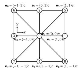
Figure 1. D2Q9 Cartesian lattice and discrete velocities.
