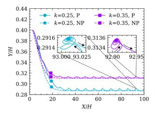
**Figure 7.** The particle center trajectory for k = 0.25 (two sky-blue curves with circle marker), k = 0.35 (two purple curves with square marker) at Re = 50. Solid curve represents the case driven by pulsatile velocity, which is abbreviated as P, while NP is the acronym for non-pulsatile flow donated by dash curve.
