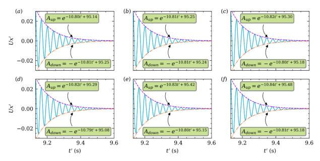
**Figure 11.** Damping of  $U'_x$  at Re = 50 and different = (**a**) 0.15, (**b**) 0.20, (**c**) 0.25, (**d**) 0.30, (**e**) 0.35, (**f**) 0.40. Envelope curves are fitted in the same way.
