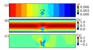
**Figure 6.** The contour view of (**a**) the dimensionless pressure p', (**b**) the dimensionless fluid velocity in X direction  $U'_x$  and (**c**) in Y direction  $U'_y$  in stable state of particle migrating in non-pulsatile flow at k = 0.25 and Re = 50.
