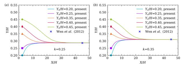
**Figure 4.** Lateral migration of the particle released from different initial positions in Poiseuille flow with (**a**) k = 0.25, (**b**) k = 0.35.
