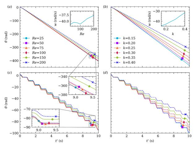
**Figure 9.** The particle orientation at different  $Re(\mathbf{a},\mathbf{c})$  and  $k(\mathbf{b},\mathbf{d})$ . Meanwhile,  $(\mathbf{a},\mathbf{b})$  is in non-pulsatile and  $(\mathbf{c},\mathbf{d})$  in pulsatile flow.
