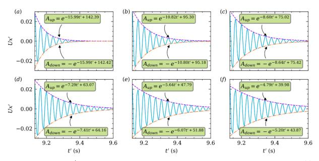
**Figure 10.** Damping of  $U'_x$  (solid line in sky-blue color) of the particle at k = 0.25 and different  $Re = (\mathbf{a})$  25, (**b**) 50, (**c**) 75, (**d**) 100, (**e**) 150, (**f**) 200. The upside (dashed line in purple color) and downside (dash dotted line in orange color) envelope curves are fitted by exponential function.
