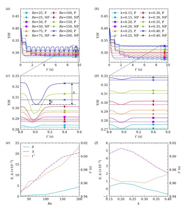
**Figure 8.** Time history of the particle center trajectory at different Re (**a**,**c**) at k = 0.25, and different k (**b**,**d**) at Re = 50. The variation of  $\delta$ ,  $\Delta$ ,  $t^*$  with Re (**e**) and k (**f**).
