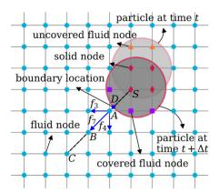
Figure 2. Improved bounce-back scheme boundary conditions. Lighter gray circle represents the location of particle at time t and darker gray circle at time  $t + \Delta t$ , which result in two orange triangles uncover to fluid node, three purple squares cover to solid node and four red thin diamonds remain solid node. The other sky-blue circles denote the fluid nodes. The distribution function  $f_7$  can be determined by the information of node S, D, A, B, C.
