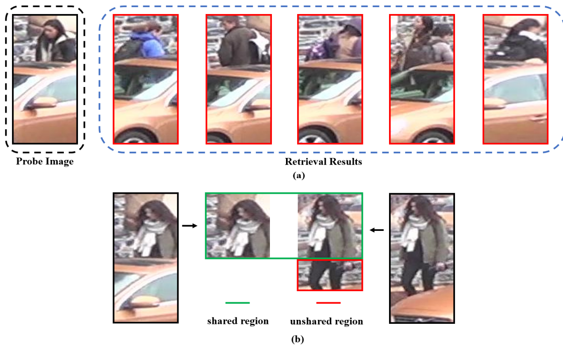
Figure 1. Two challenges of the occluded person re-identification problem. In (a), owing to the influence of obstacles, previous Re-ID methods may incorrectly retrieve the image of a similar car; in (b), the unshared regions (the red region on the right image) become distracting noises that interfere with retrieval.
