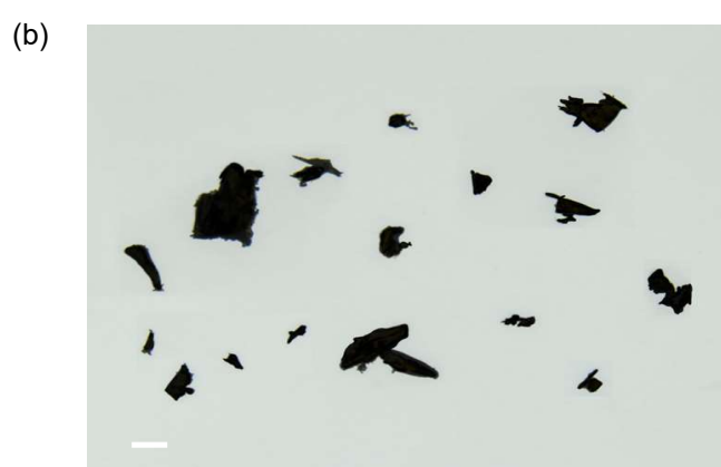
Figure S15. Photos of \text{FuBIGH}_2(\text{CO}_3)(\text{H}_2\text{O})_4 crystals under the microscope. Related to Figure 3. (a) \text{FuBIGH}_2(\text{CO}_3)(\text{H}_2\text{O})_4 crystals before heating. (b) The crystals of \text{FuBIGH}_2(\text{CO}_3)(\text{H}_2\text{O})_4 had been heated in an oven at 120^\circ\text{C} for 1h, the crystals transformed to FuBIG and changed their appearance from transparent to opaque. The scale represents 25\ \mu\text{m} .
