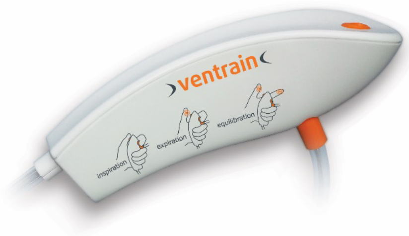
Figure 4. The Ventrain® device. This simple-to-operate manual ventilator is operated using one's thumb and index finger. It features active expiration based on the Bernoulli Principle, allowing ventilation through small-bore tubes. In addition to inspiratory (positive pressure) and expiratory (negative pressure) modes of operation, an equilibration (safety) mode is available where no significant positive or negative pressure is present at the tip of the attached ventilation catheter. The figure and text have been reproduced with permission from Ventinova Medical, Eindhoven, The Netherlands.
