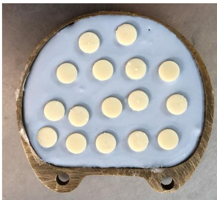
Figure 3. Wax patterns for fabricating specimens using the conventional compression-molding technique.
