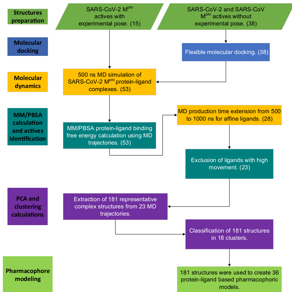
Figure 2. Summary of the methods to generate pharmacophore models for SARS-CoV-2 M pro . We collected 15 inhibitors with protein–ligand crystal available and 38 inhibitors with protein–ligand crystal unavailable. These 38 inhibitors went through a molecular docking process to predict ligand poses on the active site. The 38 predicted poses and the 15 experimental poses were taken to perform a MD simulation with 500 ns production time. The MD trajectories were used for MM/PBSA free energy calculations and 28 systems with protein–ligand binding free energy less than -100 kJ/mol were identified and the respective ligands were considered as possible actives. The MD production time of these 28 systems was extended to 1000 ns. Ligands showing prominent movement on the active site were excluded resulting in 23 actives. The 23 MD trajectories were used for a PCA and clustering process in order to extract representative conformations of each ligand on the active site. Finally, the conformations were employed to create protein–ligand-based pharmacophore models.
