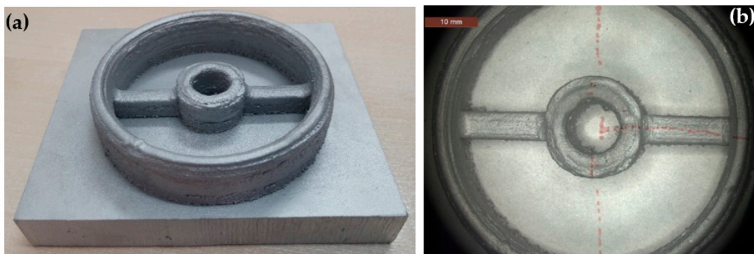
Figure 4. Deposition from scratch of a housing made of Al 4047 alloy by LENS. (a) Charge coupled device (CCD) camera view, (b) stereomicroscope view.
