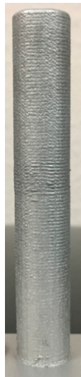
Figure 1. Macroscopic view of a 17-4 PH stainless steel rod with an approximate diameter of 1.27 cm and height of 8.18 cm that was printed by LENS.
