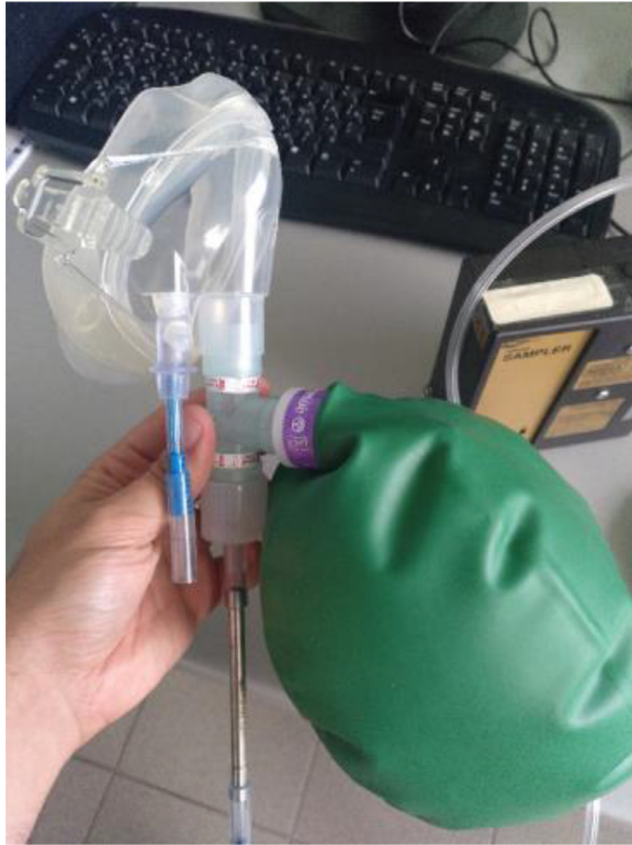
Fig. 6. Face Mask 1 tube collection system.
