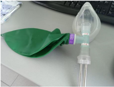
Fig. 5. Face Mask 4 tubes collection system (left); self-made TD tube connector (middle); T-piece directional valve (right).
