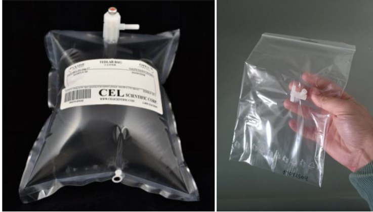
Fig. 1. Tedlar® Bag (Left) and developed Minigrip plastic bag collection system (Right).
