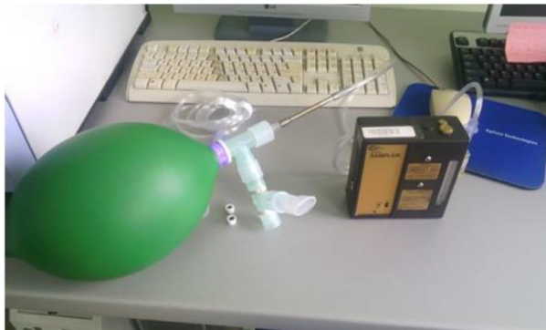
Fig. 7. Face Mask 1 tube collection system.
