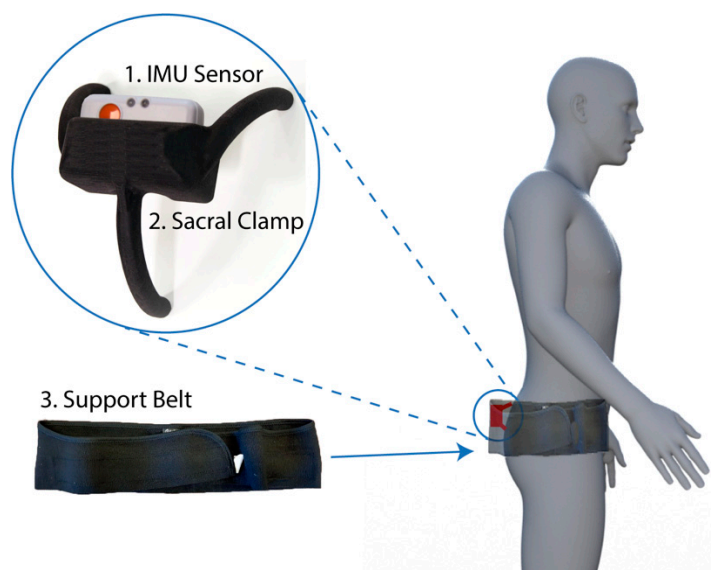
Figure 1. Device components and fitting location. The device consisted of three components: Inertial measurement unit (IMU) sensor (1), a bespoke sacral clamp (2), and support belt (3). The device was attached across the sacrum and held in place by the belt.
