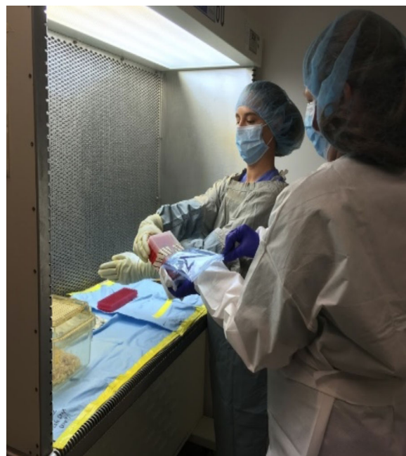
Figure 2. Material handling. The SA ( right ) must open the material wrapping so that only the sterile material is inside of the airflow and the FA's hand ( left ) does not have to exit the sterile area.
