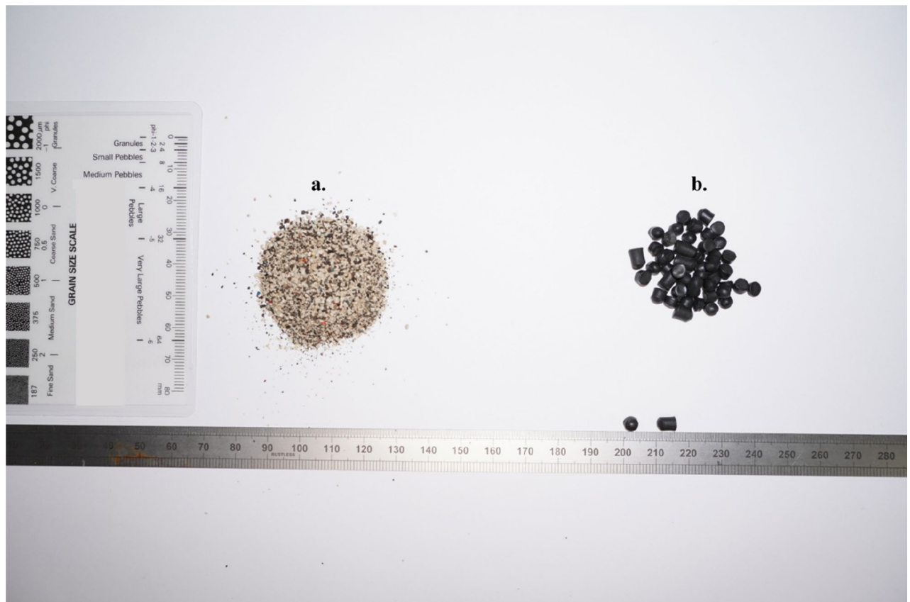
Figure 10. Microplastics, (a) Bakelite particles and (b) PVC nurdles, deployed in the experiment.
