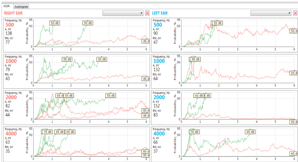
Fig. 2. Definition of ASSR threshold on an ASSR screen as a function of time (in minutes). When stimulation has been initiated, a significant response is sought for by the algorithm in all channels. If significance is reached in one of them, recording ceases in this channel (e.g. 55 dB at 2 kHz right), while it continues in the other ones. In the channel where significance was found, the stimulation resumes at a 5 dB nHL lower intensity; the routine continues until no significant response is obtained after 6 min (e.g. 45 dB nHL at 2 kHz right). Thresholds for the right ear are 50 dB nHL at 1 kHz, 55 dB nHL at 2 kHz and 65 dB nHL at 4 kHz. A = amplitude of the signal (nV); RN = residual noise.
