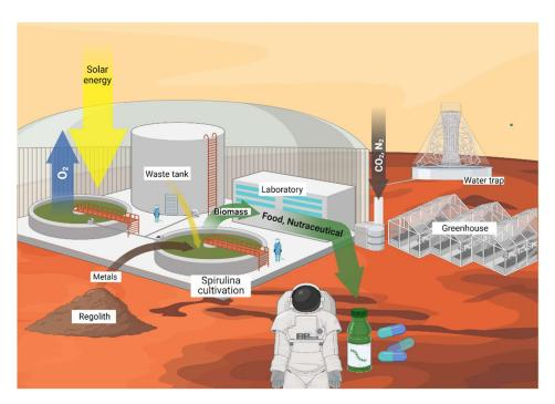
**Figure 2.** Rendering of ECLSS and ISRU systems for the cultivation and utilization of *Spirulina* on Mars. Created with **BioRender.com** (accessed on 8 March 2022).
