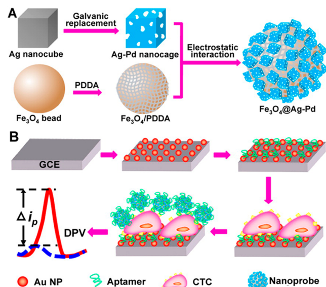
Figure 5. Schematic illustration of the fabrication of Fe 3 O 4 @Ag-Pd hybrid NPs (A) and the cytosensor assembly process (B). Reprinted from ref 205. Copyright 2014 American Chemical Society.
