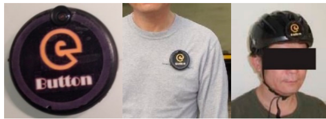
Figure 9. Appearance and two possible ways to wear the eButton device.
