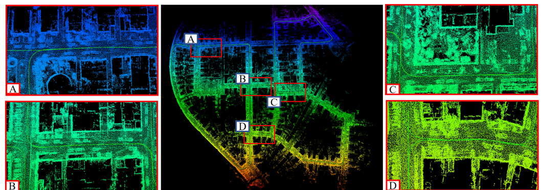
Figure 10. Our mapping result on KITTI dataset sequence 00. (A–D) are some of the loop closures found in our approach.
