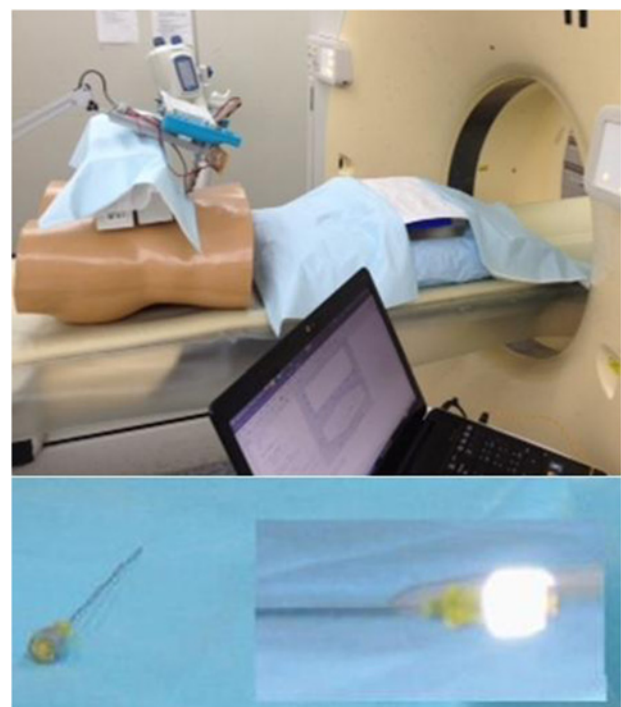
Fig. 3 Experimental setup. The CT scanner is on the right, and the IR cameras to the left
