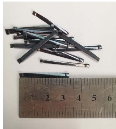
Figure 1. Mill-cut steel fiber.
