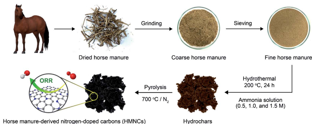
Fig. 1 Schematic illustration illustrating the synthesis of HMNCs in this work.
